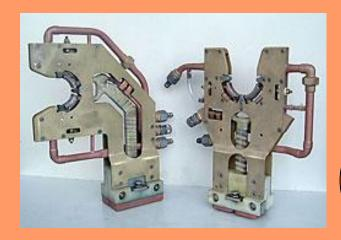
**GBZ** produces, repairs and engineers inductors for all hardening tasks, such as crankshafts and cam shafts, axis and gear components, etc.
